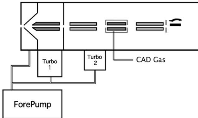
Figure 1 – Schematic of Typical API Mass Spectrometer
