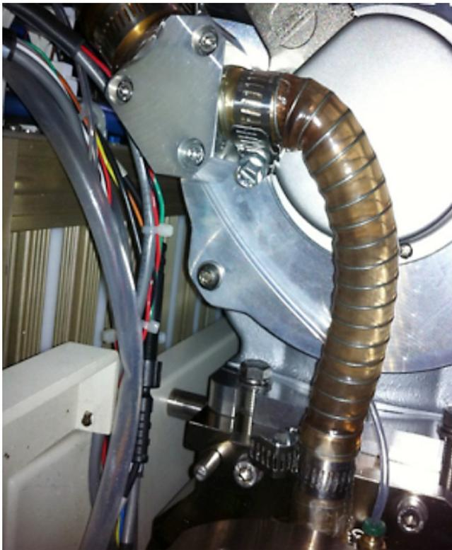
Figure 2 – Discoloration of Foreline Tubing from RVP
