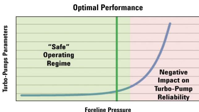
Figure 4 – Foreline Pressure Potentially Impacts Turbo- Pump Reliability
